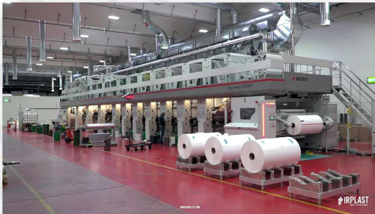
ROTOCALCO ROTOMEC 4003MP, 10 COLORI, 450m/min, FASCIA 1300mm
